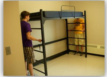
Step 3 With two or more people, grasp ends of upper unit and place onto lower unit fully seating connecting pins into bed ends. Place mattress and safety rail on spring.
