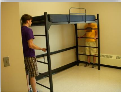
Step 1 Remove mattress and safety rail from spring. With two or more people, grasp ends of upper unit and lift up to fully remove from connecting pins from lower bed ends. Place bed on floor.
